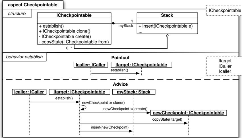
Fig. 5. The Independent *Checkpointable* Aspect (after weaving of *Copyable*)
