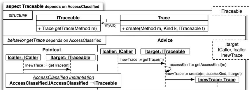
Fig. 7. The Traceable Aspect
