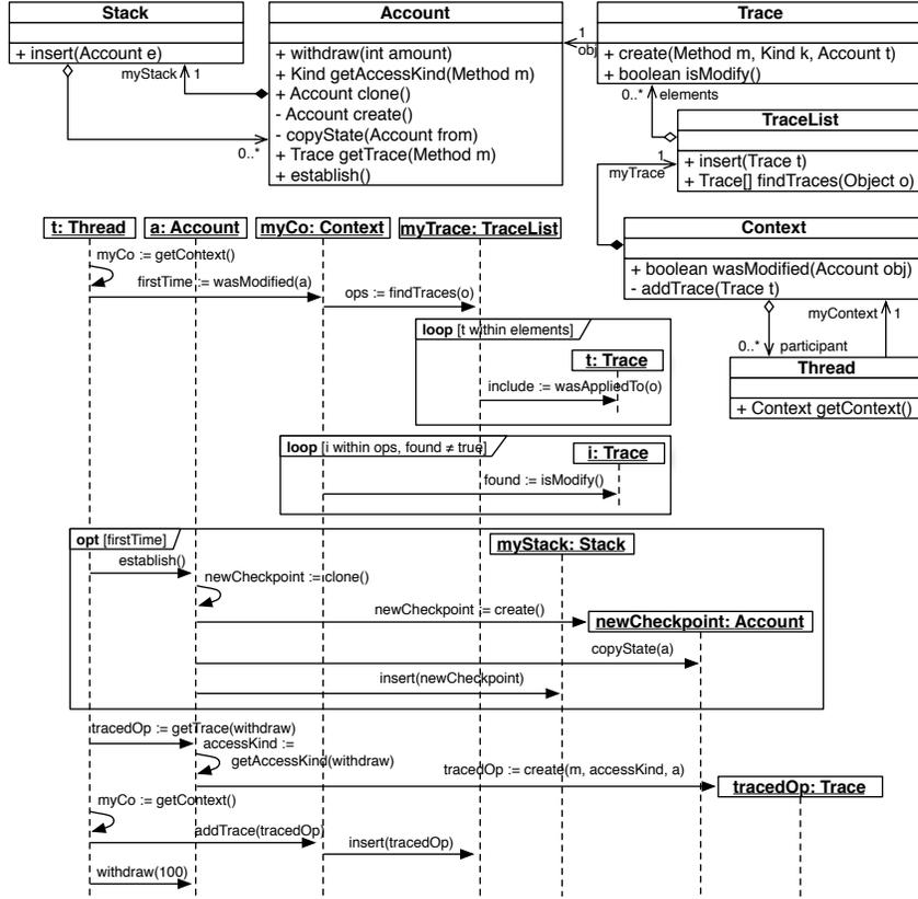
Fig. 11. Application Model after applying *Checkpointing*
